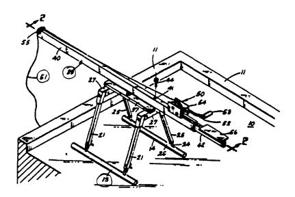
The Figure 1 depiction in the Beduhn et al patent is of a rotary crane having lift means 26 and counterbalancing weights 23, shown below:
