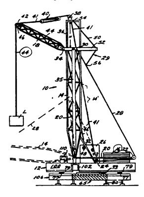
The Maxeiner patent illustrates a collapsible roof crane having a boom 2 with a lift means at one end and a counterweight support 6 at the other, and a stationary support 3, as in Figure 1 below:
