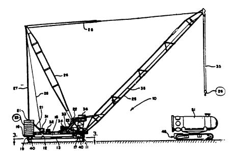
The Wilson patent describes a rotary crane with lift means 44 and counterweights 16 shown by Figure 1 below:
