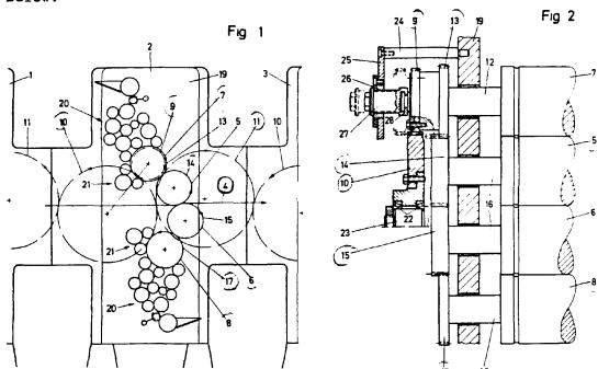
Each unit has main cylindrical drive gears 10, 11. Gear 10 drives cylindrical gear 9 to provide the only driving connection with one of the second cylindrical gears 13, 17, which are connected to separated plate cylinders 7, 8 respectively. Printing cylinders 5, 6 are in mutual contact to permit a web 4 to pass therebetween and each includes a first gear 14, 15 for engagement with gears 13, 17 respectively.
