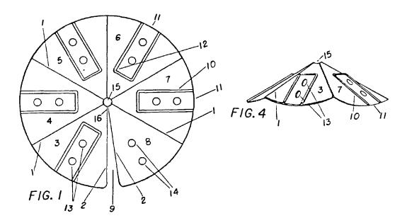
Wedge-shaped gap 9 and the flexibility of the plate allow the sectors containing holes 14 and 13 to move to align the holes (figure 4) when used for building purposes. On the face of each of the surface sectors (3-7) a three sided ridge (10) serves to locate struts which are retained by bolts through the holes in each ridge member.
