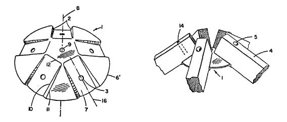
A plurality of channels (7) with sloping edges (10,11) are sized to firmly grasp struts (4) when bolt (5) is tightened.
