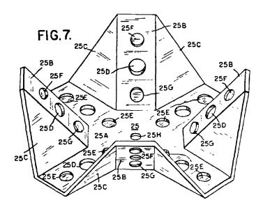
Circular coined projections (25F, 25G) match recesses in metal struts which are bolted in position through hole 25D.
