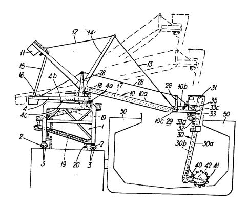
Twin bucket wheels 41 load material on conveyor 42 from which it is transferred to bucket elevator 30b and eventually reaches lowering conveyor 19.
