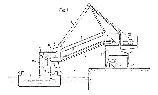
Gantry 3 has a boom system hinged to upper part 4. This boom system carries the conveyers 17, 14, 15 and bucket wheel 13.
