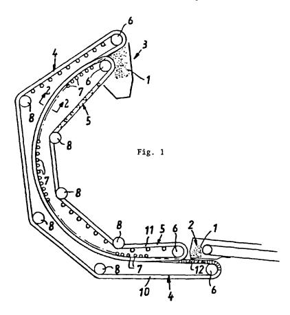
Material 1 is placed on belt 4 at 12 and is moved between belts 4 and 5 to be discharged in overhead hopper 3.
