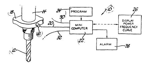
Apparatus 10 comprises a transducer 16 mounted on collar 18 in contact with drill 12, which is linked with computer 22.
