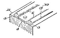
The Abbott patent relates to an insulated electrical conductor construction.
