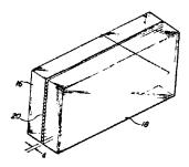
The Schemmel patent relates to an electric wire conduit consisting of a pair of electrical wires arranged in spaced parallel relationship and attached to a tape. The edges of the tape are folded over the wires and are secured to the exposed portion of the tape between the wires. Figure 3 below of the patent illustrates that invention:
