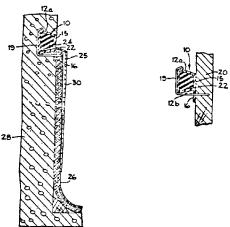
The apron 15 can be severed at 22 for insertion of the flashing 25.
