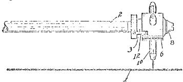
The applicant's French patent 2,151,711 relates to a spray arrangement attachable to agricultural vehicles. It consists of a boom with a number of nozzles thereon. An air chamber arrangement is used to actuate the shut-off diaphragm for each nozzle. Figure 1 of this patent is shown below.
