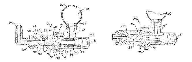
Reece discloses a turret with three jet nozzles used with Fourdrinier paper-making machines. Figure 1 of Reece appears next:
