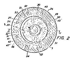
Péras and Henri-Biabaud relate to rotary engines which show that the stator has one more lobe than the rotor. Péras shows a two lobe rotor in a three lobe casing and Henri-Biabaud uses a four lobed rotor in a five lobed casing.
