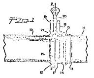
The Smith reference relates to a clamping device for holding adjacent ends of pipes in a fixed position relative to each other. Figure 1 of this patent shown below is representative of the arrangement used.
